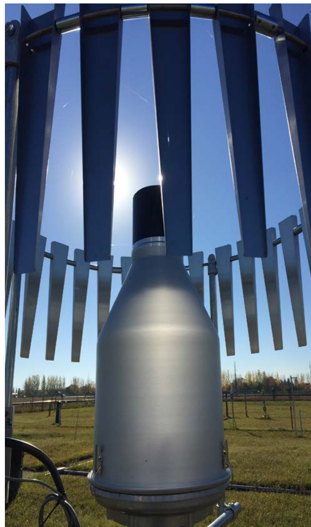
New precipitation weighing gauge 8 October 2015 Photo: V. Wittrock
