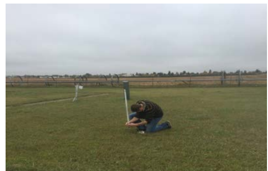
Installing Meter Sticks for Manual Snow Depth Measurements 1 October 2015 Photo: V. Wittrock
