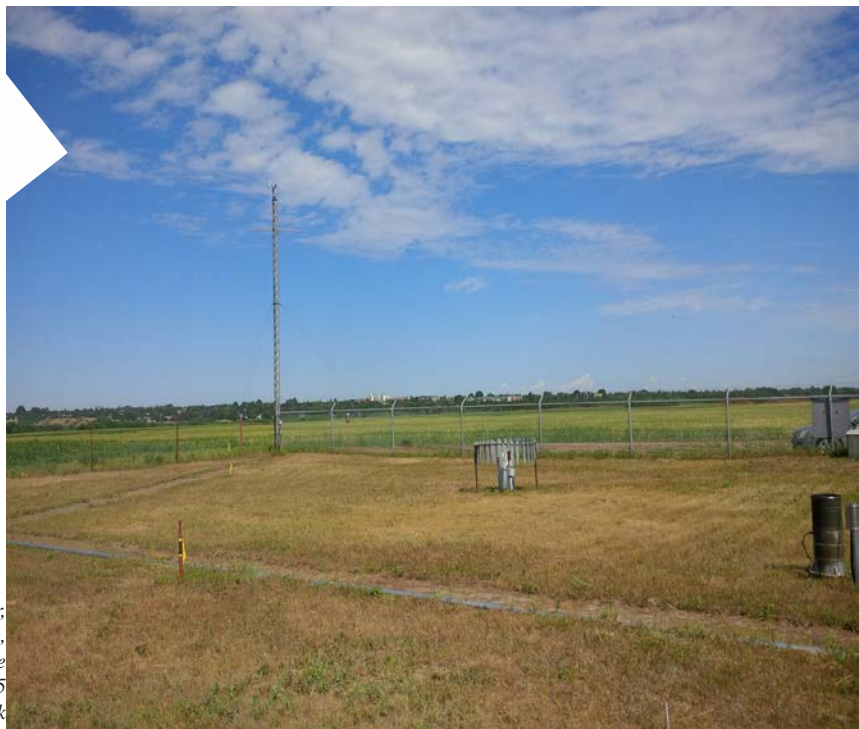
10 metre wind tower, All Season Precipitation Weighing Gauge, Tipping Bucket Gauge 15 July 2015 Photo: V. Wittrock
