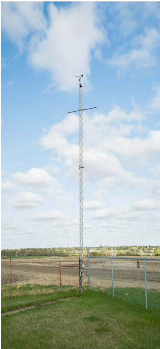
10 Metre Tower with Wind Speed and Direction May 2015 photo: E. Thiessen
