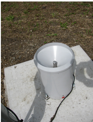
Tipping Bucket 12 July, 2011 photo credit: V. Wittrock
