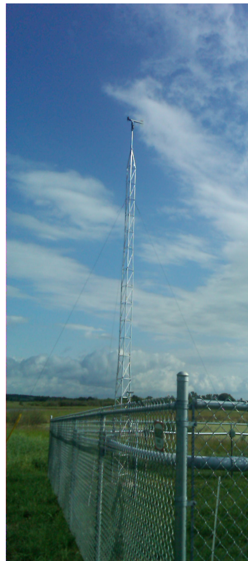
Anemometer and 10 meter tower 31 July 2012 Photo: V. Wittrock
