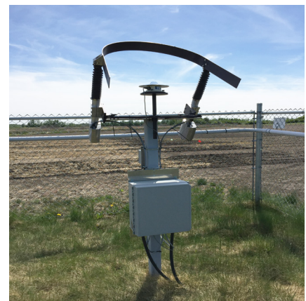
Diffuse Radiation Sensor and Automated Sunshield 3 June 2015 photo credit: R. Jansen
