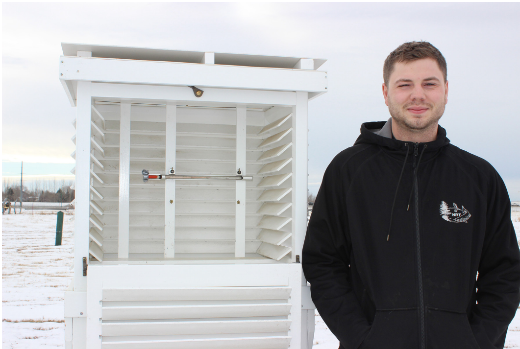
Stevenson Screen with minimum thermometer Shaw Dunn SRC technologist November 2013 photo credit: CR Beaulieu
