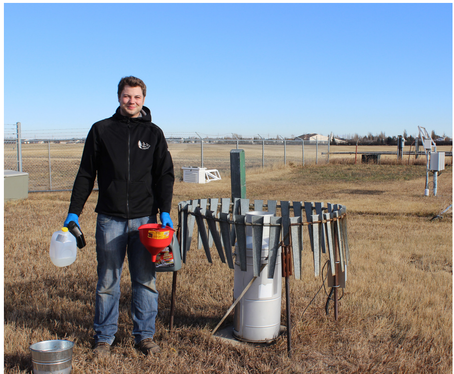
Winterizing the precipitation weighing gauge Shaw Dunn, SRC technologist, Autumn 2013 photo credit: CR Beaulieu
