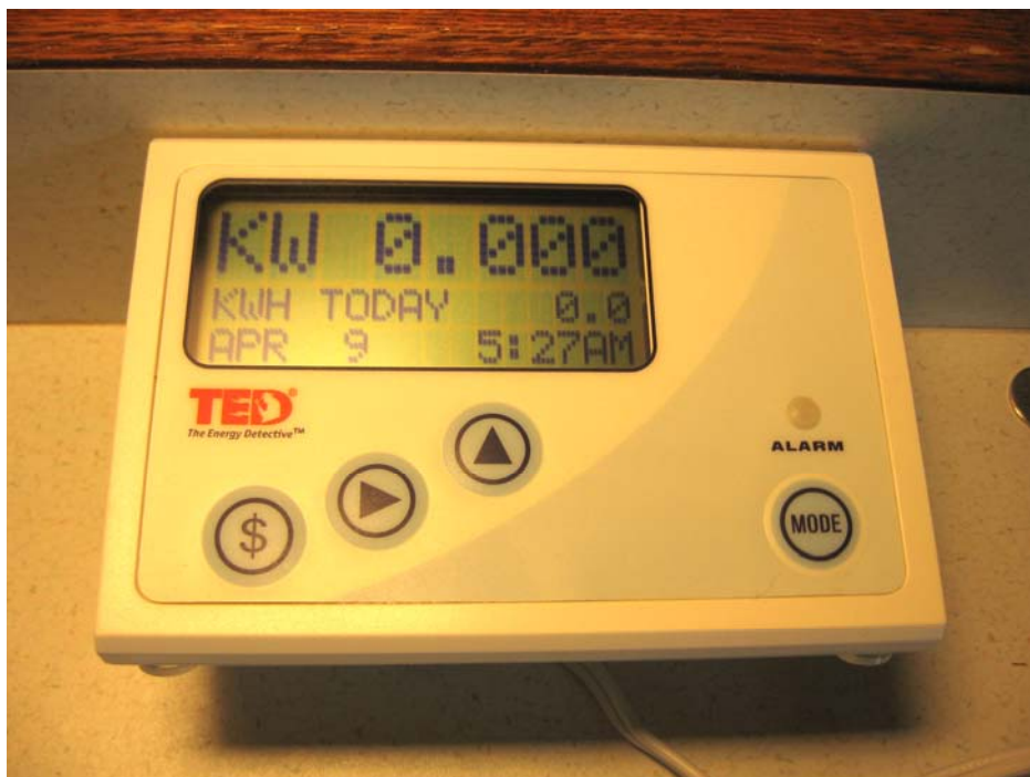
Figure 45: The Energy Detective™ instantaneous readout device
