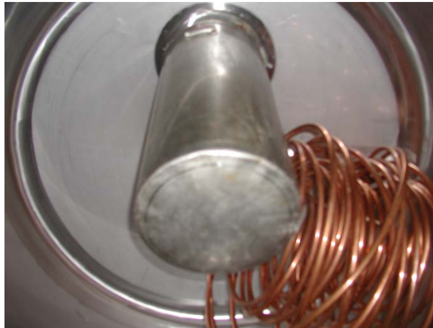
Figure 17: Small stainless steel tank and copper coil heat exchanger
