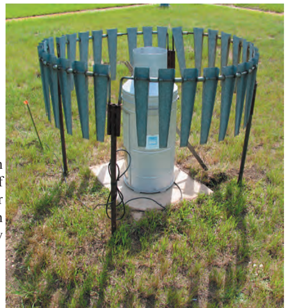
Belfort Weighing Gauge, 2005 photo credit: K. Potter
