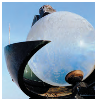
Campbell-Stokes Bright Sunshine Recorder Used at CRS from 1965-1992 photo credit: CR Beaulieu, 1993
