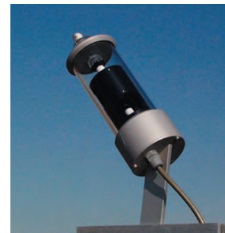
Kipp & Zonen Auto Bright Sunshine Recorder Used at CRS from 2001 to present phot credit: CR Beaulieu, 2000
