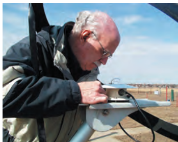
Brett Smith remounting the Global and Diffuse pyranometers after calibration, April, 2005 photo credit: CR Beaulieu
