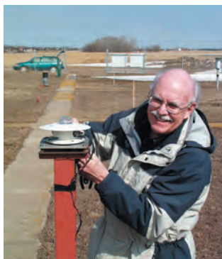
Brett Smith remounting the Global and Diffuse pyranometers after calibration, April, 2005 photo credit: CR Beaulieu
