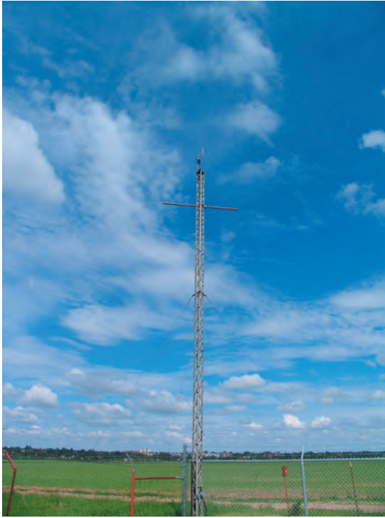
10 m tower for wind measurements at CRS, 2005. photo credit K. Potter
