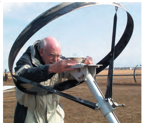
Brett Smith checking the Diffuse pyranometer after re-calibration, 2005 photo credit: CR Beaulieu, 2005
