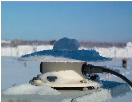
Hoar Frost on the Diffuse Pyranometer
