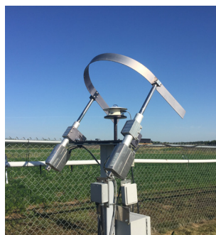
Left: Diffuse Radiation Pyranometer with auto shadow band Middle: Global Radiation Pyranometer Right: Bright Sunshine 28 July 2017 photo credit: V. Wittrock
