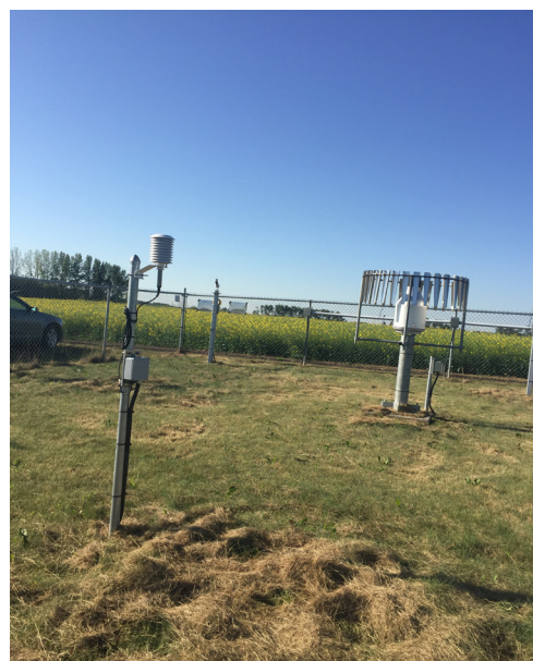
Temperature and Relative Humidity sensor and all-season precipitation gauge 28 July 2017 Photo: V. Wittrock
