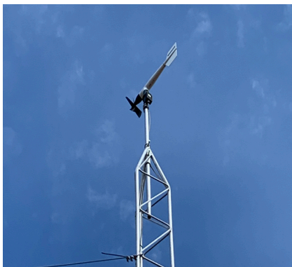
RM Young Wind Speed and Direction (10 meter height) May 2020 Photo: Development Engineering and Manufacturing
