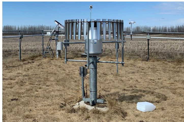
All-season precipitation weighing gauge with anemometer at 2 meter height May 2020 Photo: Development Engineering and Manufacturing
