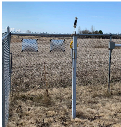
Soil Moisture Sensors wire conduit sealed May 2020 Photo: Development Engineering and Manufacturing
