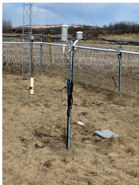
Duplicate air temperature / relative humidity sensors May 2020 Photo: Development Engineering and Manufacturing
