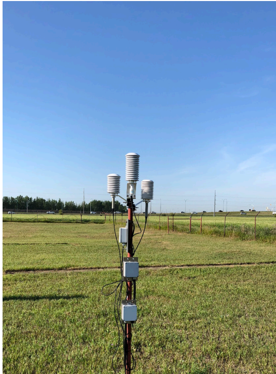
Temperature and Relative Humidity Sensors (automated) July 2020 (Photo: V. Wittrock)
