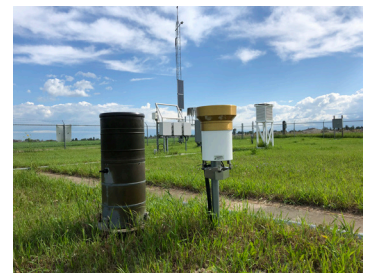
New tipping bucket for rainfall July 2020 Photo: V. Wittrock
