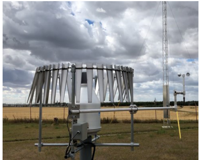
All-Season Precipitation Weighing Gauge with 2 meter anemometer 01 September 2020 Photo: V. Wittrock
