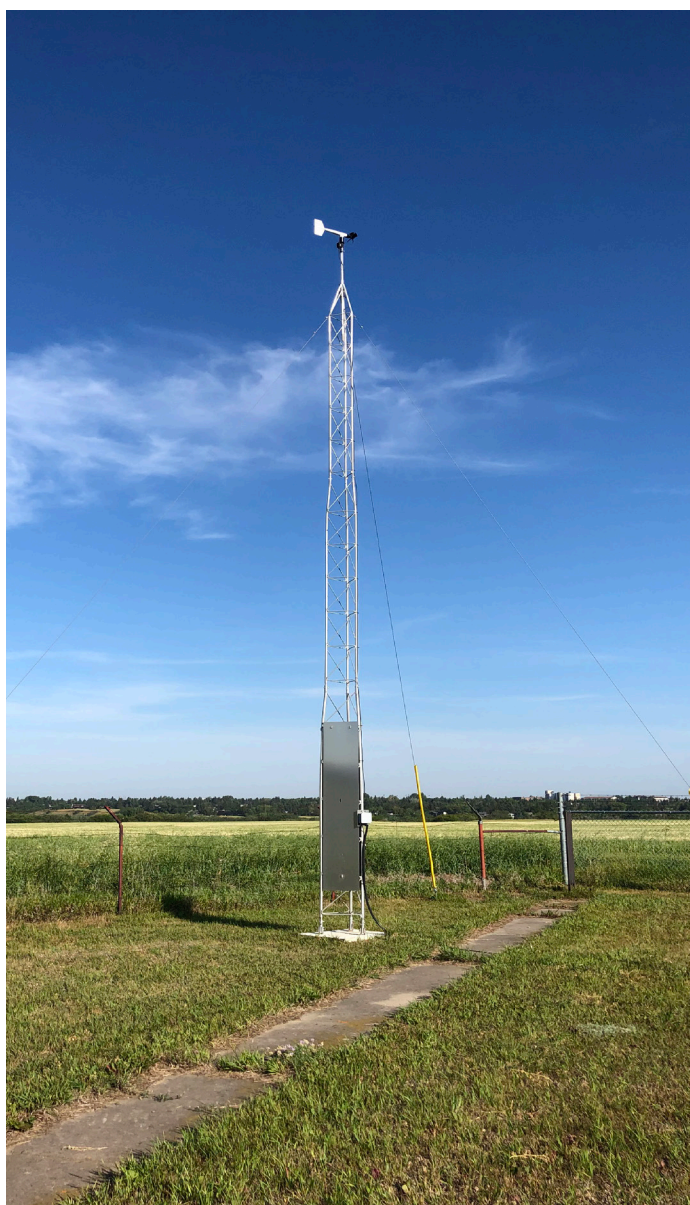
10 Metre Tower with Wind Speed and Direction 30 July 2020 photo: V. Wittrock
