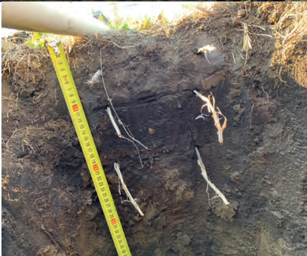
Duplicate soil temperature sensors (5, 10, 20 and 50cm depths) May 2021 Photo: R. Jansen
