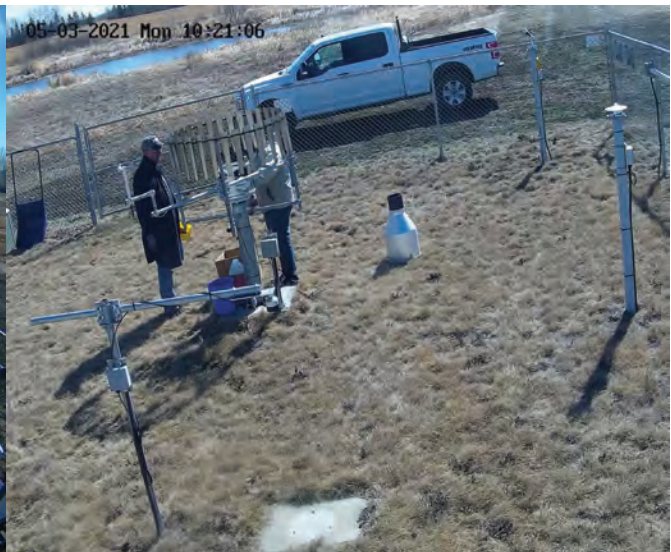
05-03-2021 Mon 10:21:06 Geonor all-season precipitation gauge spring maintenance May 2021 Photo: Camera at site
