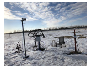
Automatic Diffuse Radiation Ring 11 March 2021 Photo: V. Wittrock
