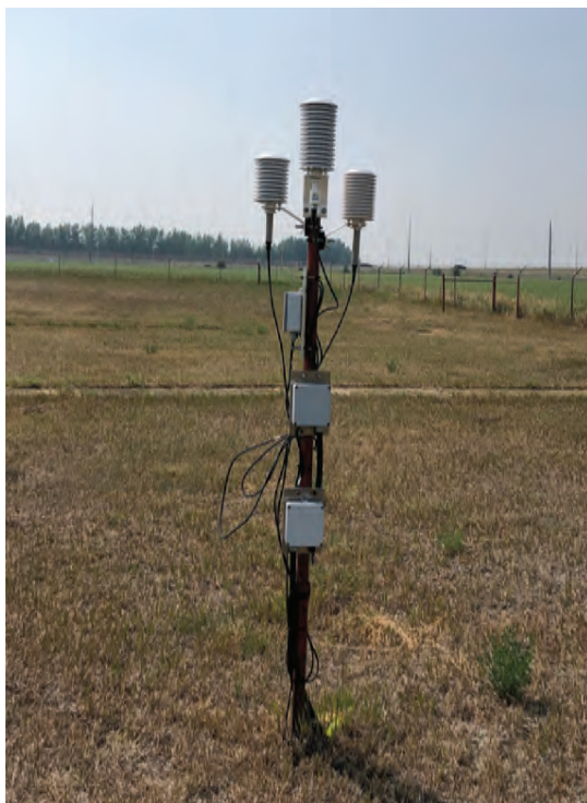
Temperature and Relative Humidity Sensors (automated) July 2021 (Photo: V. Wittrock)
