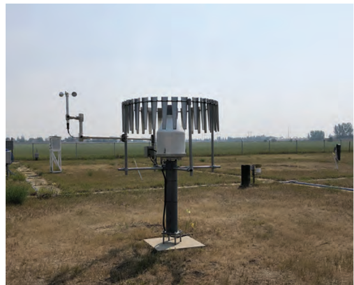
All-Season Precipitation Weighing Gauge with 2 meter anemometer 13 July 2021 Photo: V. Wittrock
