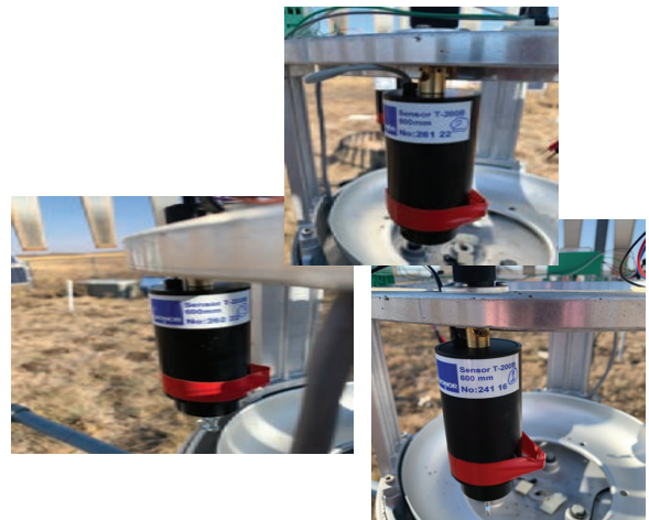
Geonor all-season precipitation gauge transducer replacement (all three) October 2022 Photo:K. Babich
