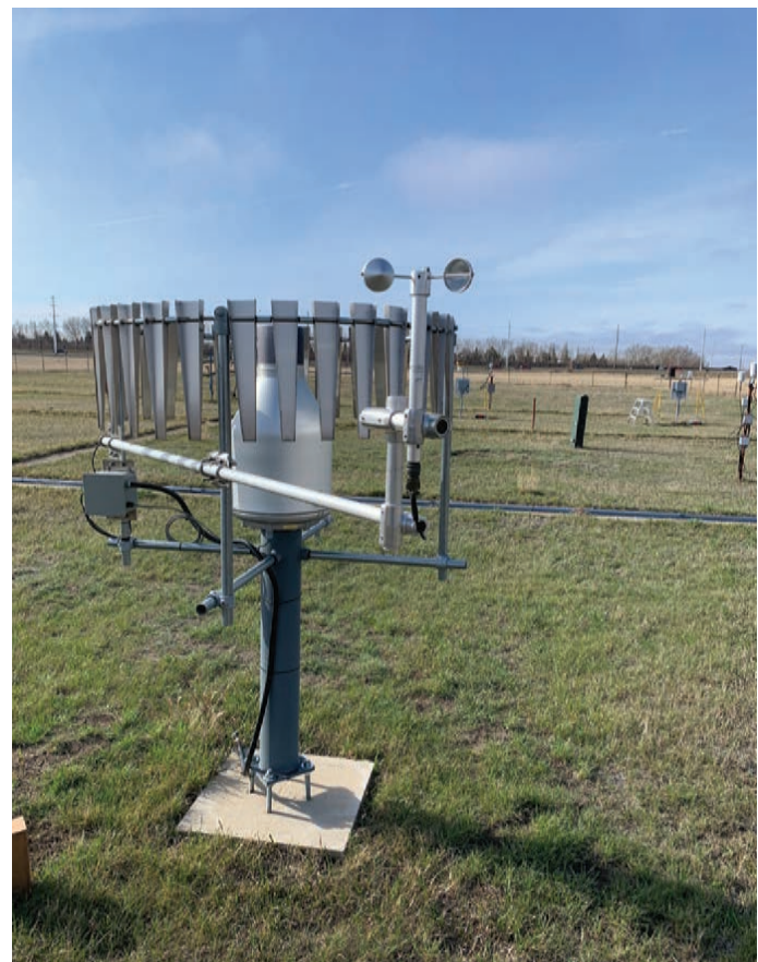
All-Season Precipitation Weighing Gauge with 2 meter anemometer 04 May 2022 Photo: G. Epp/K. Babich
