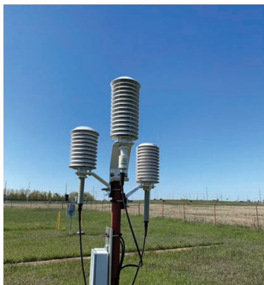
Temperature and Relative Humidity Sensors (automated) May 23 2022 (Photo: V. Wittrock)
