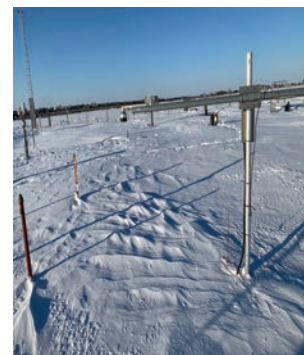
Automated Snow Depth Sensor 03 February 2022 Photo: R. Jansen
