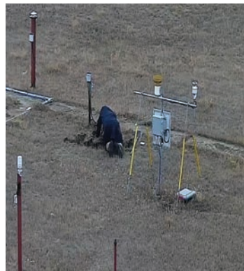
Installing replacement 10 cm soil moisture sensor October 2022 Photos: V. Wittrock
