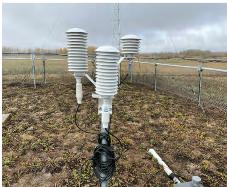
Air temperature / relative humidity sensors Oct 2023 Photo: G. Epp
