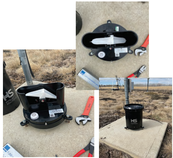
Tipping Bucket liquid precipitation gauge April 28 2023 Photo:G. Epp
