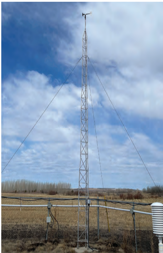
10 meter wind speed and direction tower April 2023 Photo: G. Epp
