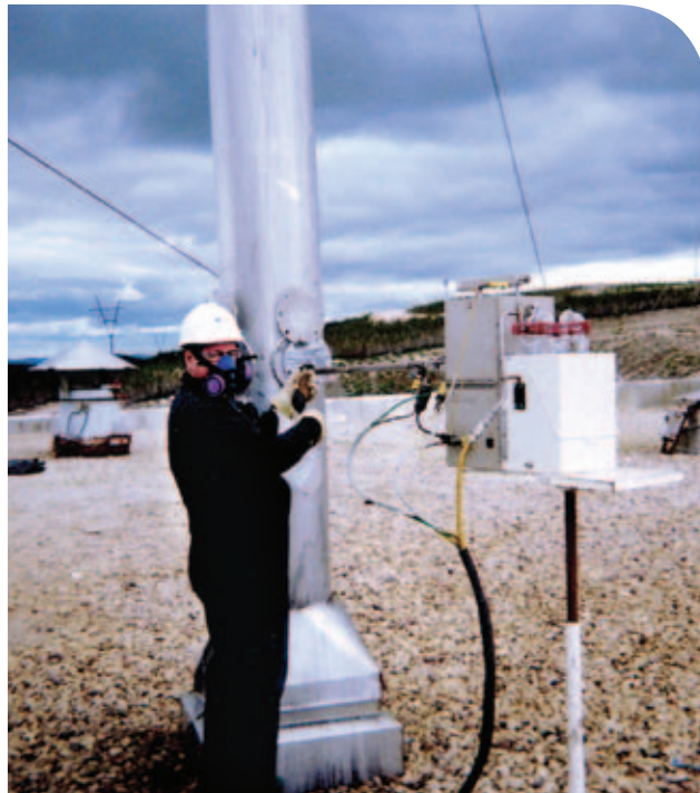
above: An example of the stack sampling train used to collect particulate and gaseous emissions from a stack.
