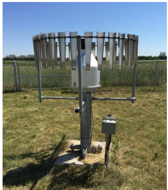
Weighing gage 28 June 2016 photo credit: R. Jansen
