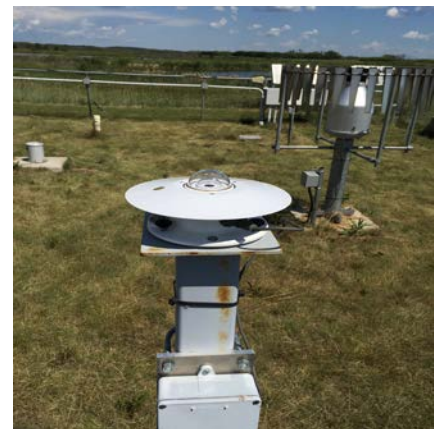
Global Radiation Sensor 16 Dec, 2015 photo credit: R. Jansen
