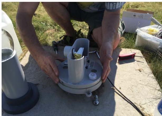
Tipping bucket Replacement 28 June 2016 Photo: R. Jansen
