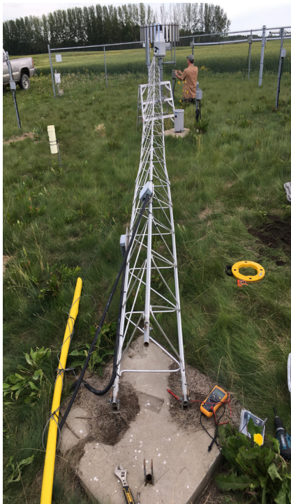
Changing bearings in 10m RM Young Aug 2018 Photo: Development Engineering and Manufacturing
