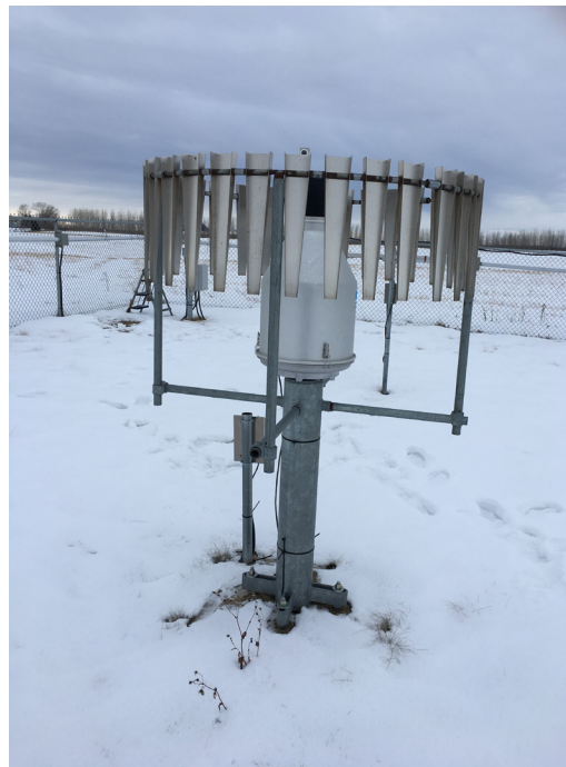
All-season precipitation weighing gauge January 2018 Photo: Development Engineering and Manufacturing
