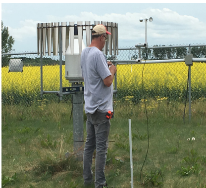
Cup anemometer placed at 2 meter height to measure wind speed July 2019 Photo: Development Engineering and Manufacturing
