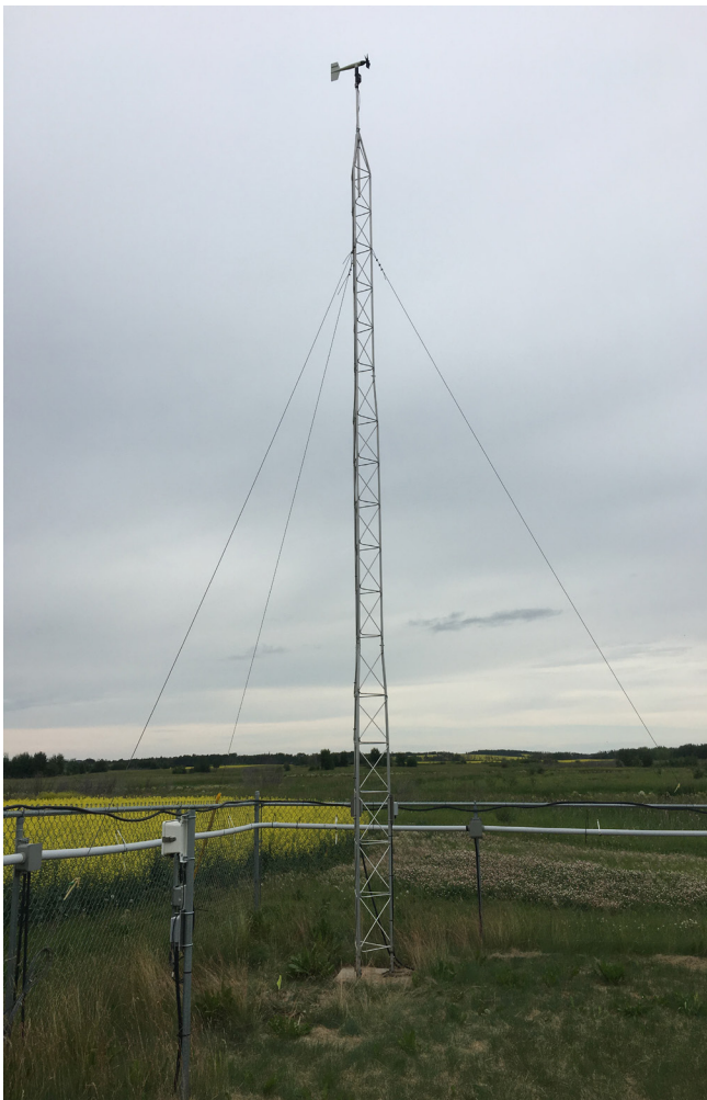
10 meter wind speed and direction tower July 2019 Photo: Development Engineering and Manufacturing
