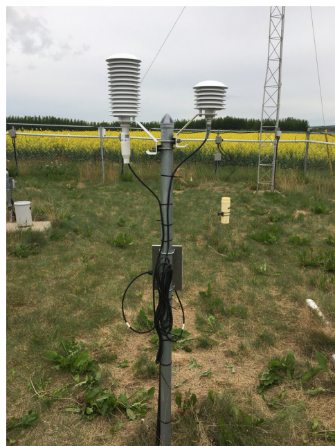
Duplicate air temperature / relative humidity sensors July 2019 Photo: Development Engineering and Manufacturing
