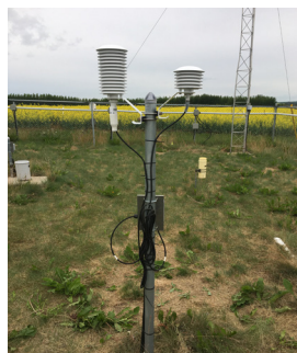
New air temperature sensor July 2019 Photo: Development Engineering and Manufacturing
