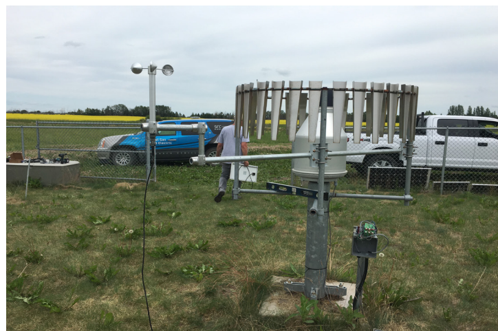
All-season precipitation weighing gauge with anemometer at 2 meter height July 2019 Photo: Development Engineering and Manufacturing
