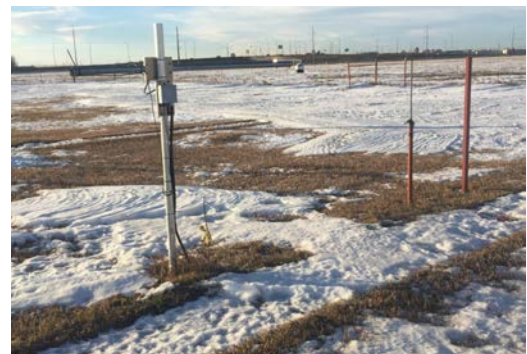
Automated Snow Depth Sensor and Discontinuous Snow Cover 12 December 2017 Photo: V. Wittrock
