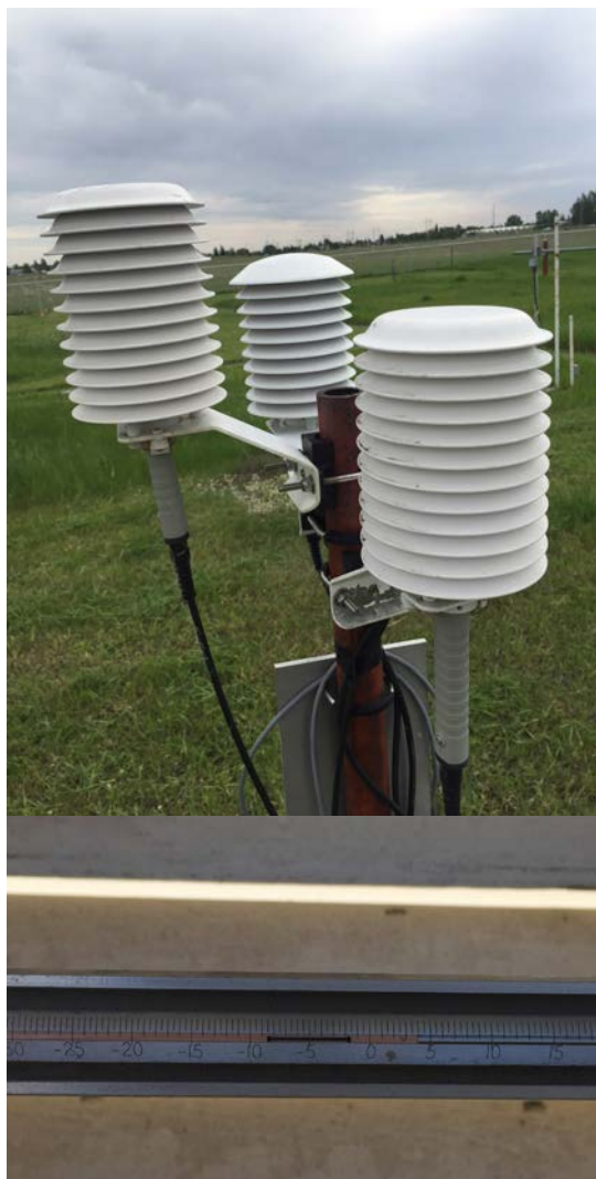
Top - Temperature and Relative Humidity Sensors (Automated) June 2017 (Photo: J. Janzen) Bottom - Minimum thermometer housed in Stevenson Screen (first fall frost temperature reading on 4 Oct 2017) (Photo: V. Wittrock)
