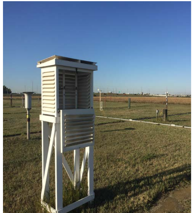
Stevenson Screen that houses the Minimum Manual Thermometer 06 September 2017 Photo: V. Wittrock
