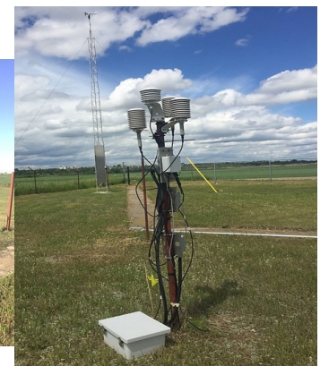
Calibrating Air Temperature Sensors June 2018 Photo: V. Wittrock
