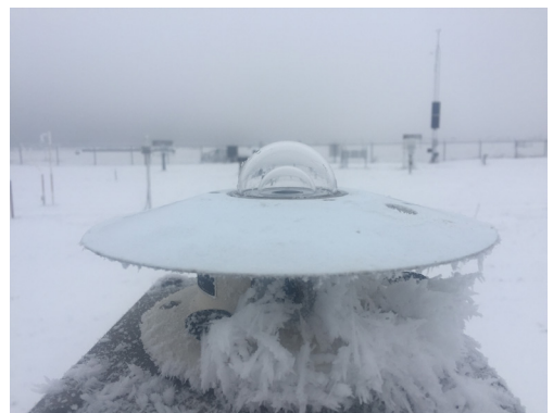
Global Radiation Pyranometer (left with Rime Frost; Right Rime frost cleared off 30 Nov 2018 Photo: V. Wittrock
