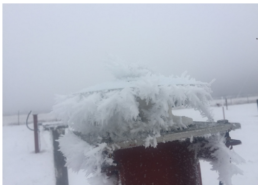
Global Radiation Pyranometer (left with Rime Frost; Right Rime frost cleared off 30 Nov 2018 Photo: V. Wittrock
