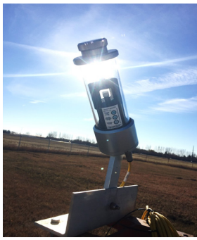
Recalibrated bright sunshine - installed 12 April 2018 Oct 2018 Photo: V. Wittrock
