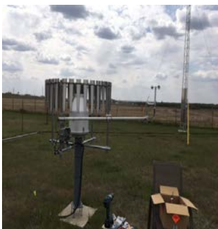
2 meter cup anemometer added to all season precipitation gauge May 2019 Photo: V. Wittrock
