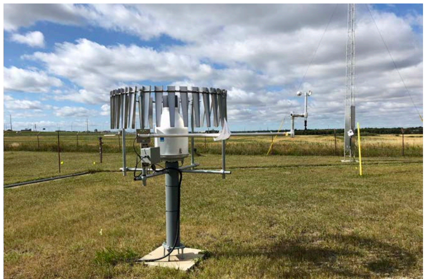
All-Season Precipitation Weighing Gauge with 2 meter anemometer 05 September 2019 Photo: V. Wittrock
