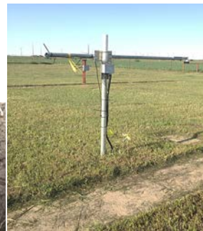
Snow Depth Sensor maintenance Nov 2019 Photo: V. Wittrock
