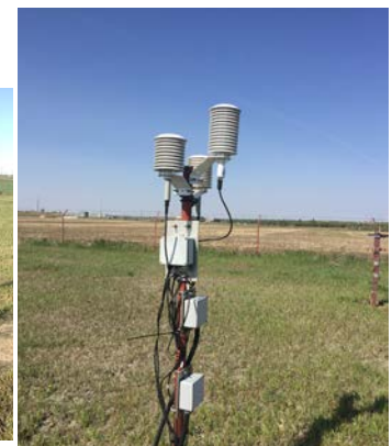
Added HMP 155 Air Temperature & RH sensor (calibrated for -80 to +60C) to temperature array May 2019 Photo: V. Wittrock
