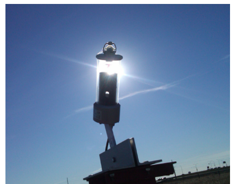
Kipp and Zonen bright sunshine recorder photo credit: V. Wittrock
