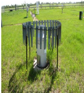
Belfort Weighing Gauge May 2014 Photo: V. Wittrock
