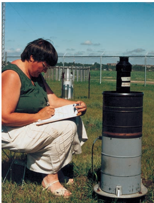
C. Beaulieu calibrating tipping bucket Circa 2000 Photo: SRC
