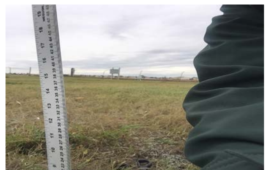
Installing Meter Sticks for Manual Snow Depth Measurements 3 October 2016 Photo: V. Wittrock
