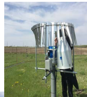
All-Season Precipitation Gauge General Maintenance May 2016 Photos: V. Wittrock
