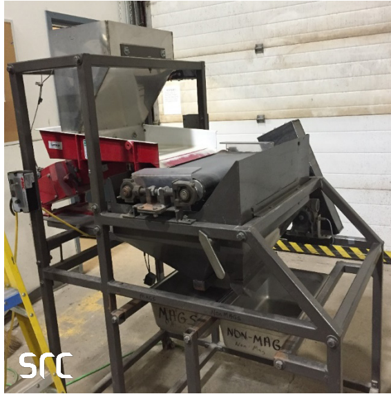
One-stage magnetic separator at SRC
