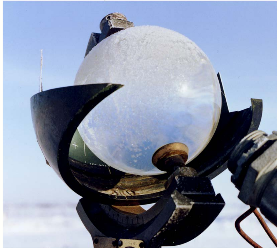
Campbell-Stokes Bright Sunshine Recorder. CRS Saskatoon, c 1993 photo credit CR Beaulieu
