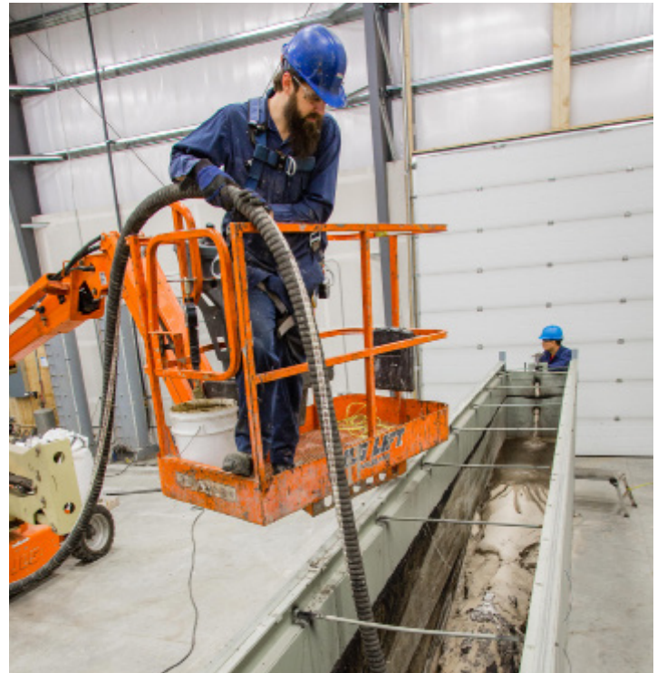
Large open channel flume in the Tailings Test Facility
