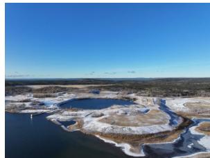
Pic 2: Rip Rap places in the shore of Langley Bay Tailings cover
